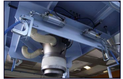
INFLATABLE FILL SPOUT
